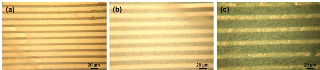
Figure. 8.6. Optical microscopy images of S/D patterns with (a) 5 \mu\text{m} (b) 10 \mu\text{m} and (c) 20 \mu\text{m} length after the deposition of ZnO by drop-casting.
